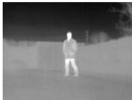
Figure 6: Thermal imaging from an uncooled microbolometer camera can enhance VISWIR images for self-radiating objects
