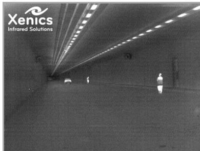
Figure 6: Seeing through smoke IR
