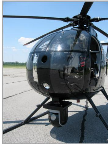
*Stabilized Gimbal with smart thermal camera combination*
